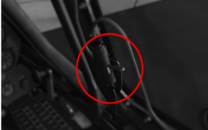
Cockpit Pressure Valve
