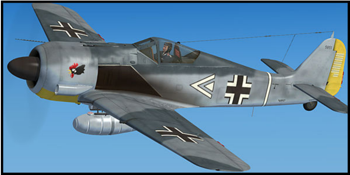
Fw 190 A-4"U7" of Hauptmann Egon Mayer, Kommodore of III./JG 2, early 1943. Note the external engine air intakes.
