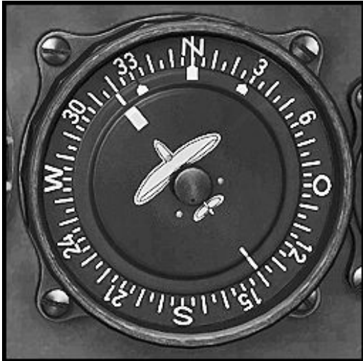
Heading Indicator FL.23334 electrically driven slave
