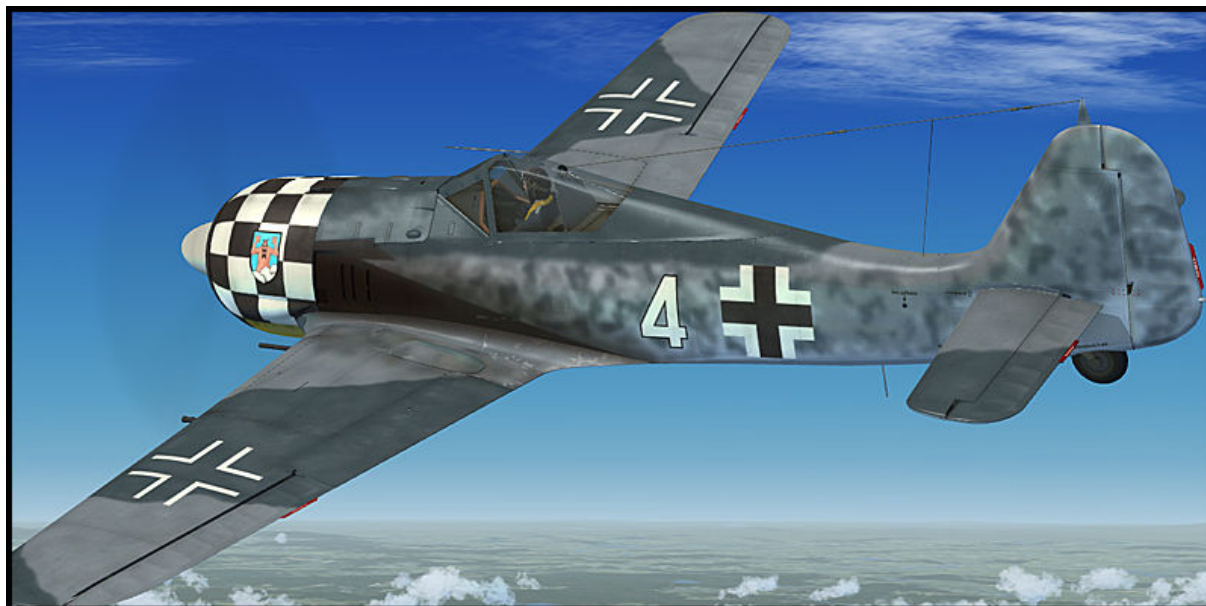
Fw190A-4 of I./JG 1, Schiphol, Netherlands, June 1943. This aircraft is still equipped with the fixed cooling slot, the so-called 'Kiemenspalten'.
