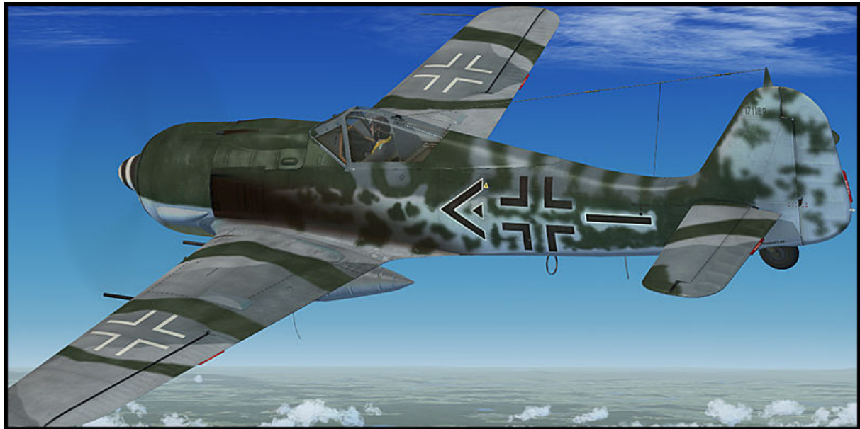
Fw190A-8 of Major Karl Kennel, Kommandeur of II./SG 2, Mai 1945. Note the Mk 108 blisters on top of the wings, indicating that this aircraft had provision to carry either Mk 108 or Mg 151/20 cannons.
