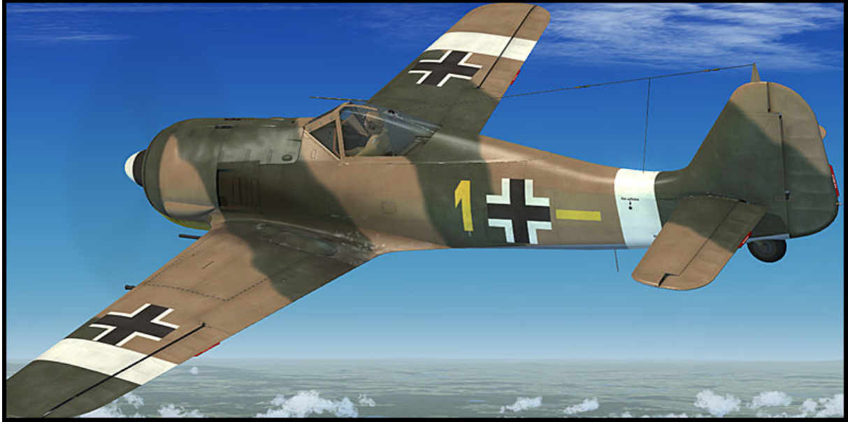
Fw 190 A-4 of Erich Rudorffer, 6./JG 2, Tunisia, early 1943. This aircraft has the adjustable cooling flaps installed. One of the rare examples of the Tunisian campaign that actually received desert camouflage.
